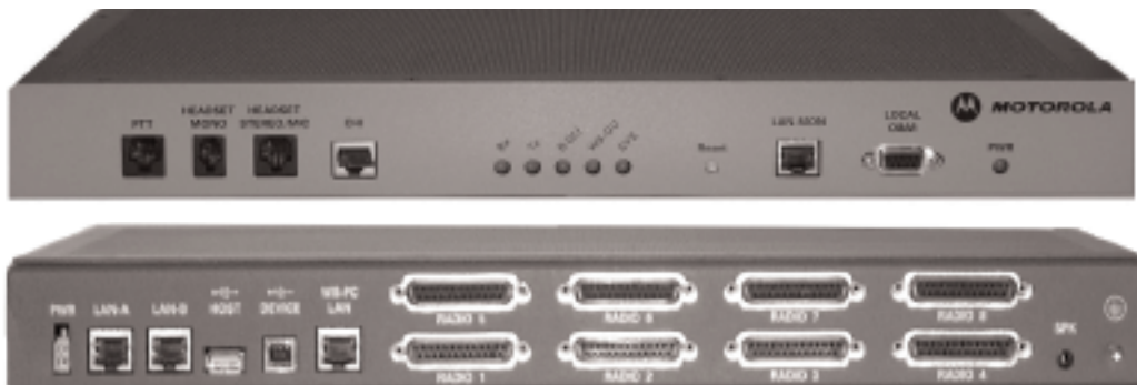
Front and back view of Gateway Unit (RGU or WSGU)
